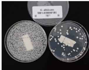
Figure 8 Result of test population control group and test group against C. albicans for 48 hours
